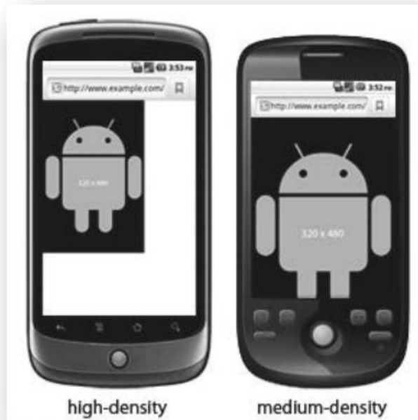
Figura 2 Viewport =device – width y target –densitydpi = device – dpi.
